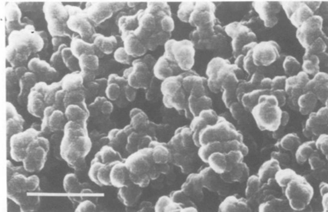
Figure 2-5. Scanning electron micrograph of Sephacryl<sup>®</sup> S-500<sup>7</sup>. The white bars represent 10  $\mu\text{m}$  (top picture) and 0.5  $\mu\text{m}$  (lower picture). (Preparation and photo: A. Medin, Department of Biochemistry, Uppsala University, Uppsala, Sweden).
