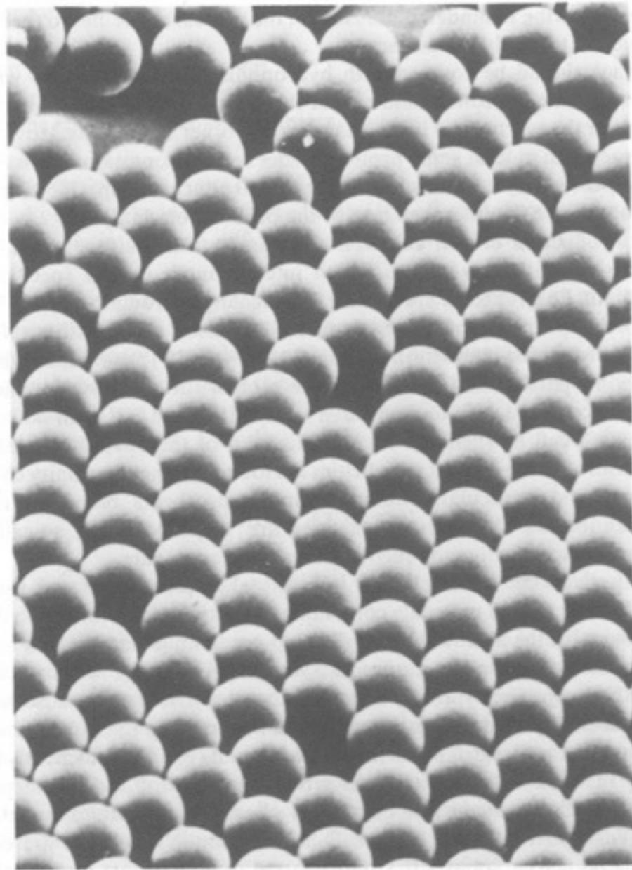
Figure 2-6. Scanning electron micrograph of MonoBeads™ 7.
