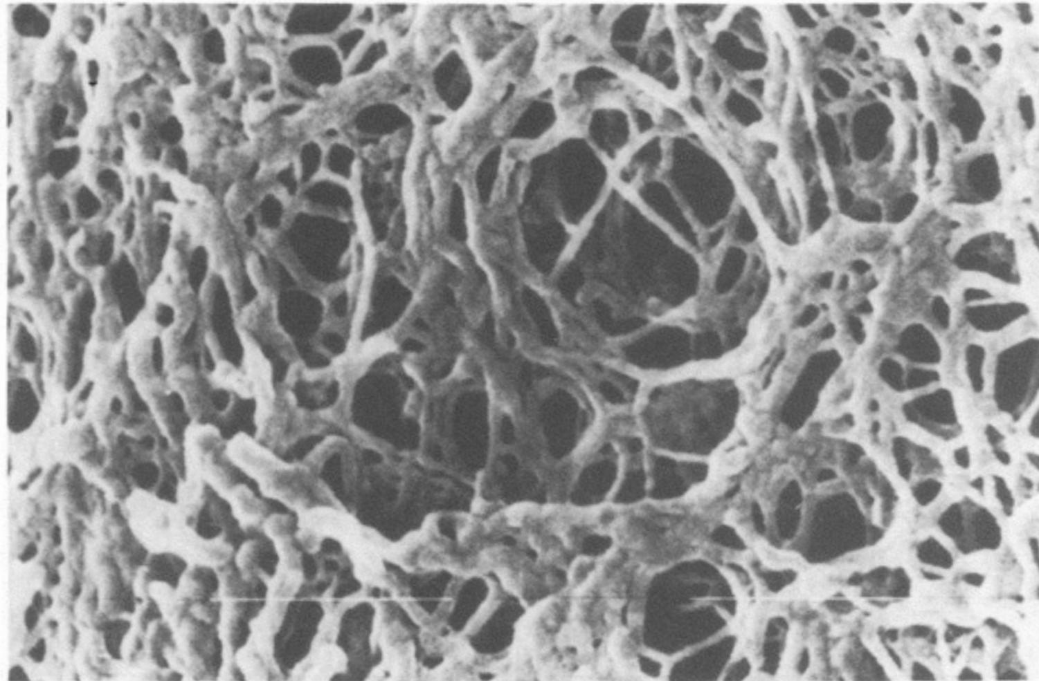
**Figure 2-4.** Scanning electron micrograph of 2% agarose gel. The white bar represents 500 nm. (Preparation and photo: A. Medin, Institute of Biochemistry, Uppsala University, Uppsala, Sweden).
